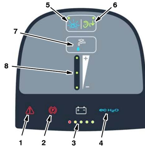
1. **Service indicator** - Lights up when a machine or charger fault is detected.
