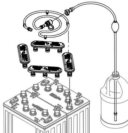
The optional HydroLINK battery watering system provides a safe and easy way to maintain the proper electrolyte levels in your batteries. It is designed exclusively for Trojan® flooded (wet) lead-acid batteries.
